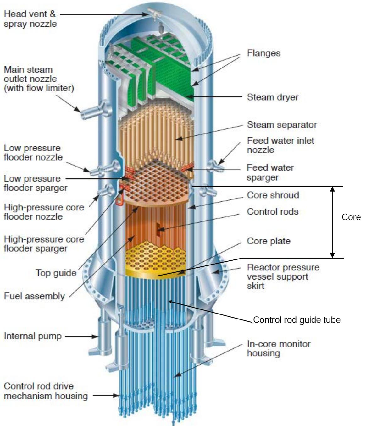
Figure 1-1 Overview of ABWR reactor
