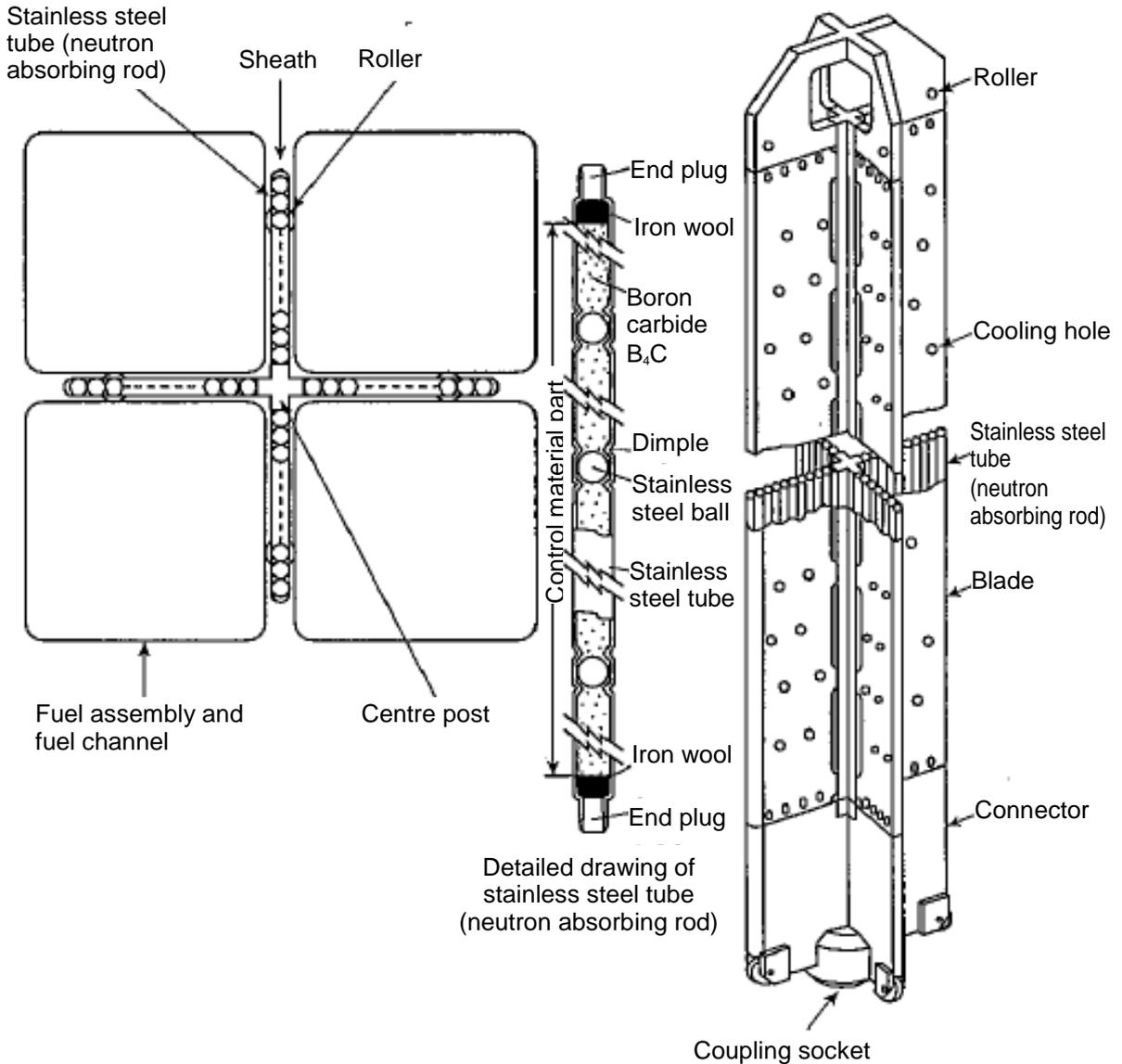
Figure 2-2 Control Rod Assembly
