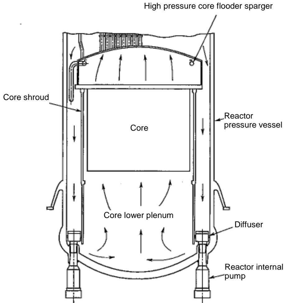
Figure 1-3 Flow of coolant in reactor pressure vessel
