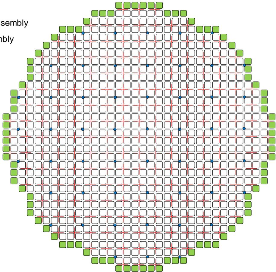
Figure 1-2 ABWR core configuration
