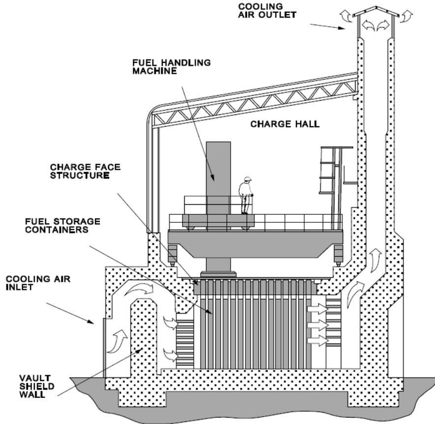
Figure 6.1.4-1 Schematic view of a modular vault dry storage (MVDS)
