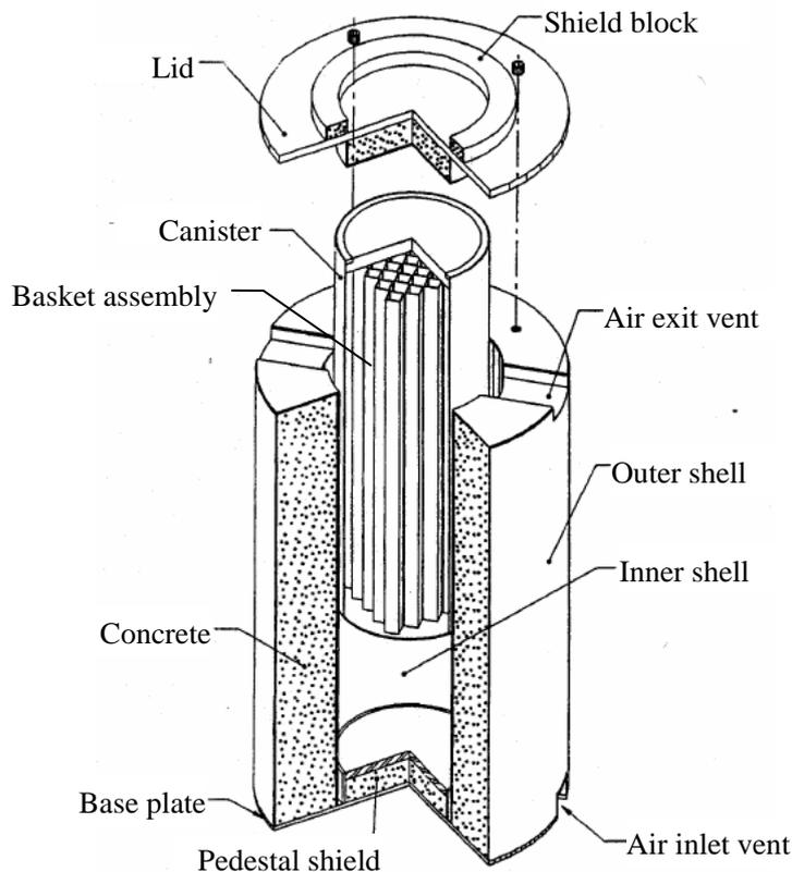
Figure 6.1.1-1 Schematic view of a typical concrete cask (Example)
