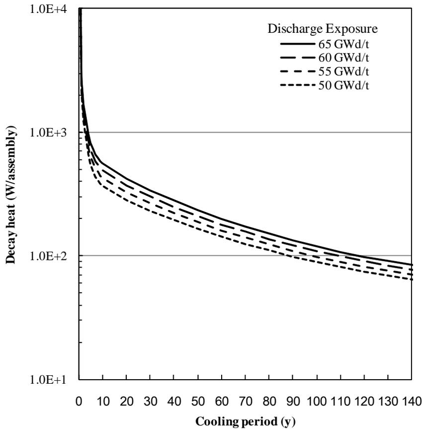
Figure 4.1-2 Transition of decay heat of GE14 spent fuel (Preliminary)
