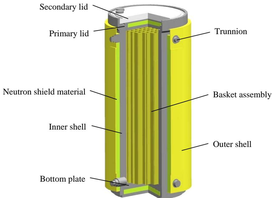
Figure 6.1.2-1 Schematic view of a typical metal cask (Example)
