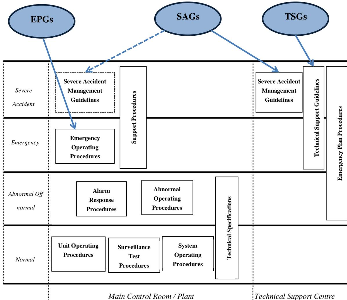
Figure 22.7-1: Operations Procedure Interactions
