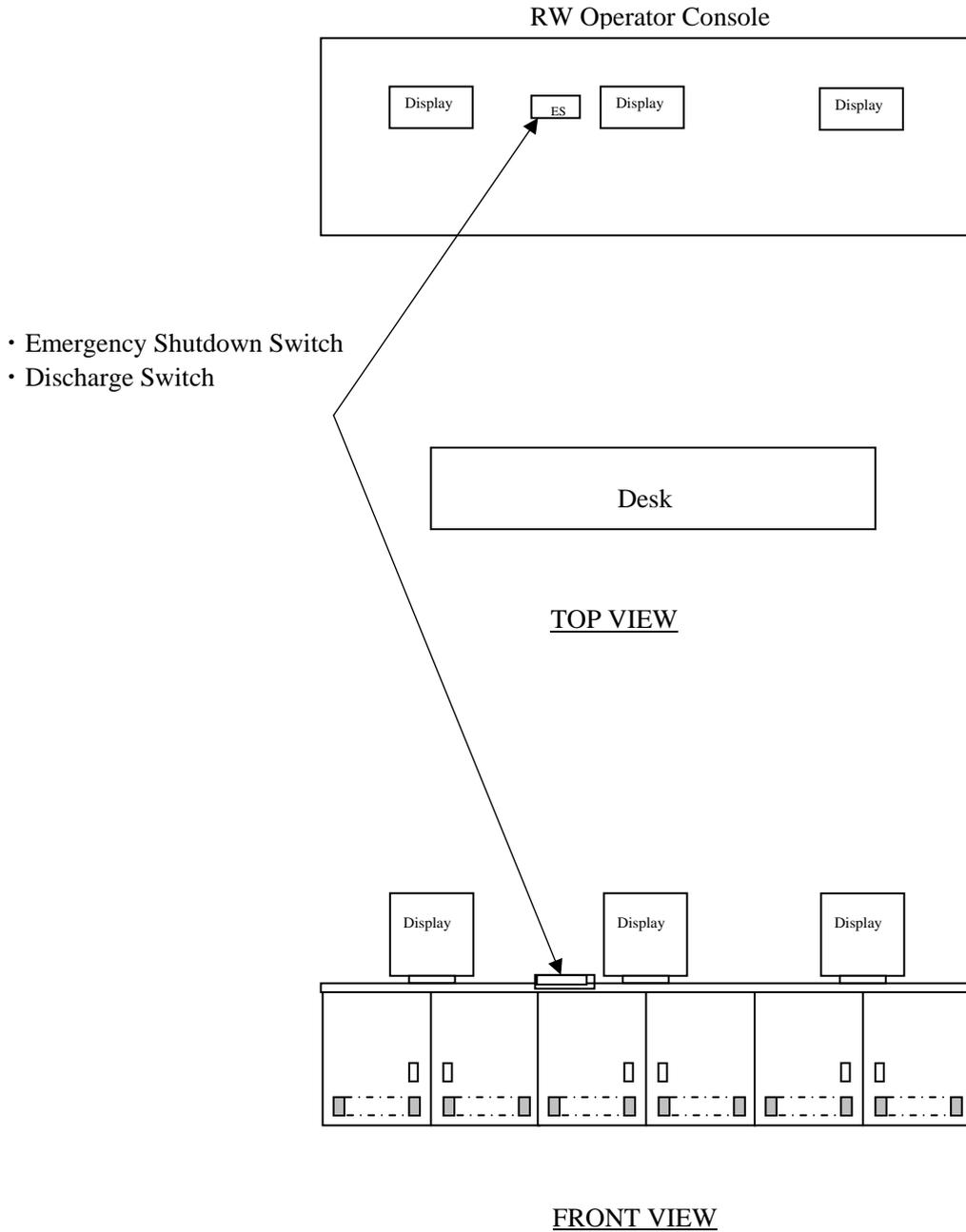
Figure 21.6-1: The Basic Layout of RW Operator Console
