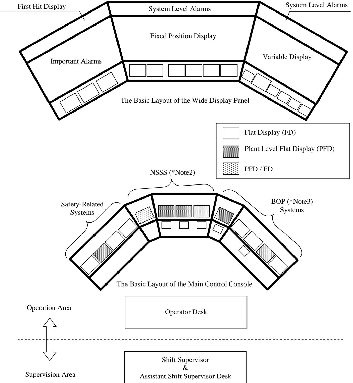
Figure 21.3-1: The Basic Layout of a MCR
