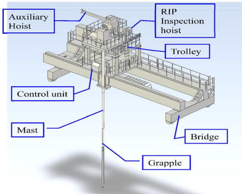
Fig.19.5-1: Schematic view of the FHM
