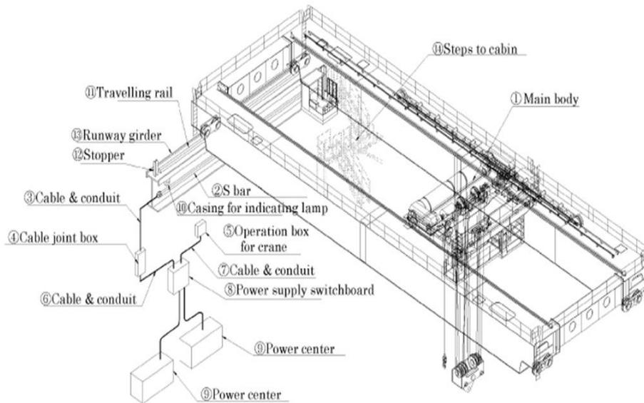
Fig.19.6-1: Schematic view of R/B Overhead Crane
