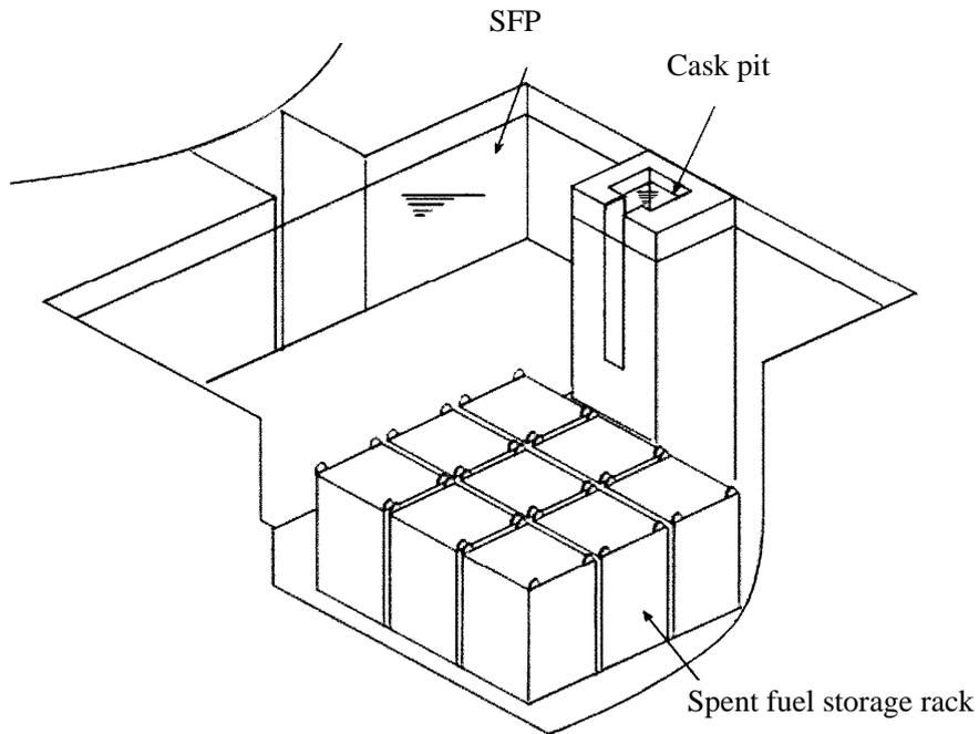
**Fig.19.3-1: Schematic view of Spent Fuel Storage**
