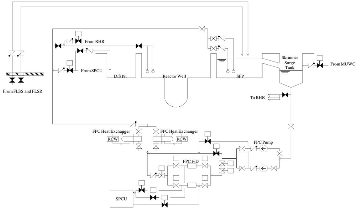
Figure 19.4-1: Outline of the Fuel Pool Cooling and Clean-up System
