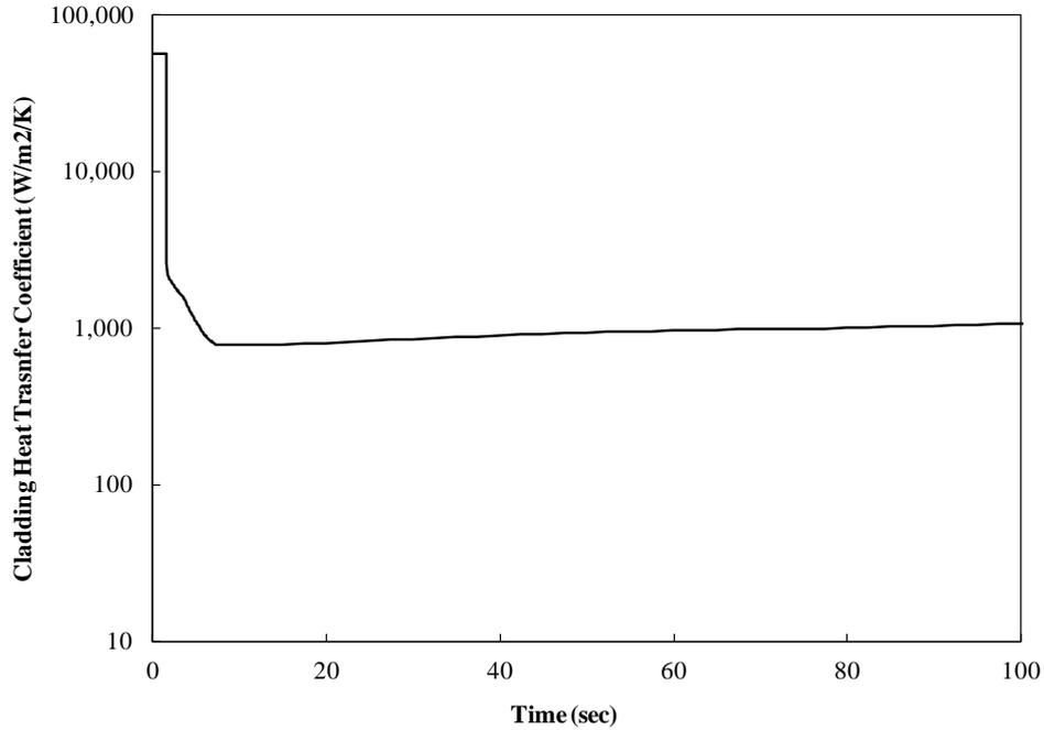
**Figure 13.3-9 : Heat Transfer Coefficient at the Position where Fuel Cladding Temperature is Maximum during the Double-ended Break Accident of HPCF Line (with actuation of RCIC, two LPFL pumps)**
