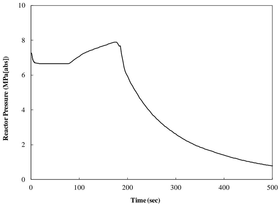
Figure 13.3-8 : Reactor Pressure during the Double-ended Break Accident of HPCF Line (with actuation of RCIC, two LPFL pumps)
