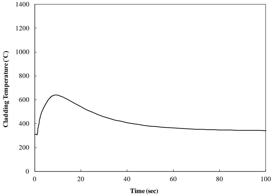
**Figure 13.3-10 : Fuel Cladding Temperature at the Position where Fuel Cladding Temperature is Maximum during the Double-ended Break Accident of HPCF Line (with actuation of RCIC, two LPFL pumps)**
