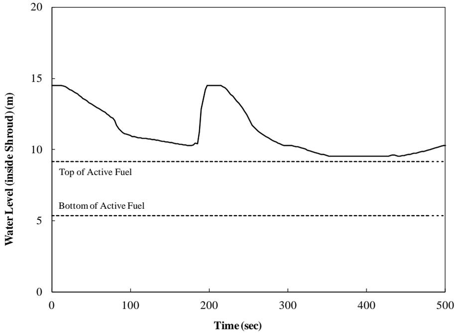
Figure 13.3-7 : Reactor Water Level during the Double-ended Break Accident of HPCF Line (with actuation of RCIC, two LPFL pumps)
